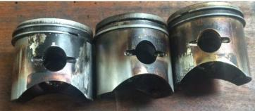
In case of engine seizure and pistons are like those in the photos, possible causes are as follows
